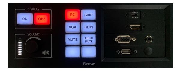
For more information on the operation of the audio and video equipment with button panel, see: <u>https://zid.univie.ac.at/en/audio-video-technology/user-guides/audio-and-video-equipment-with-button-panel/</u>
